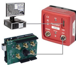
Click for Details A schematic showing a TSI-IOBOB2 connected to an Arduino in a custom camera system.
